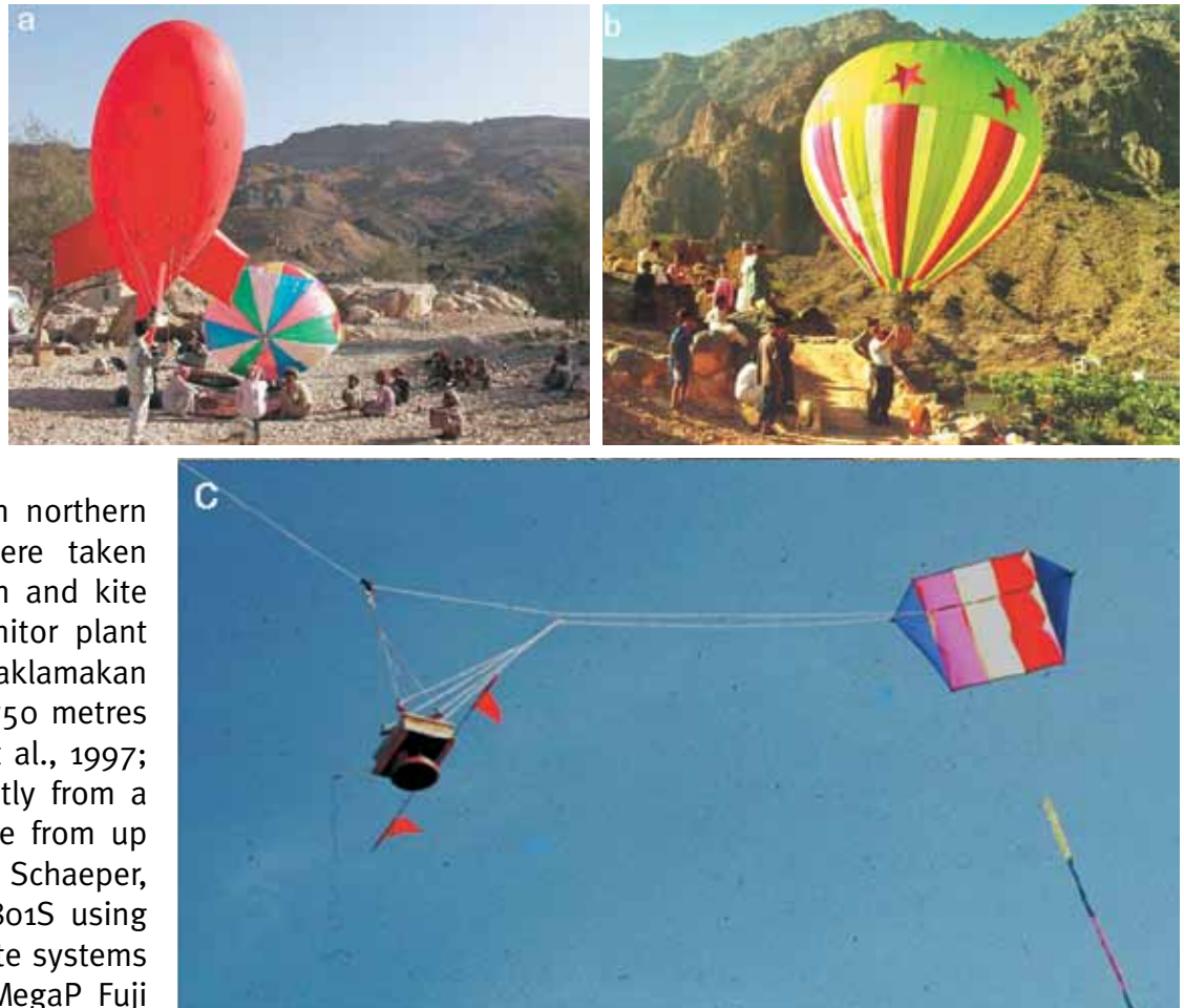
Figure 1. Helium-filled balloon (a), hot-air balloon (b) and kite system (c) used for the first low-altitude photographs of oases in Oman.
