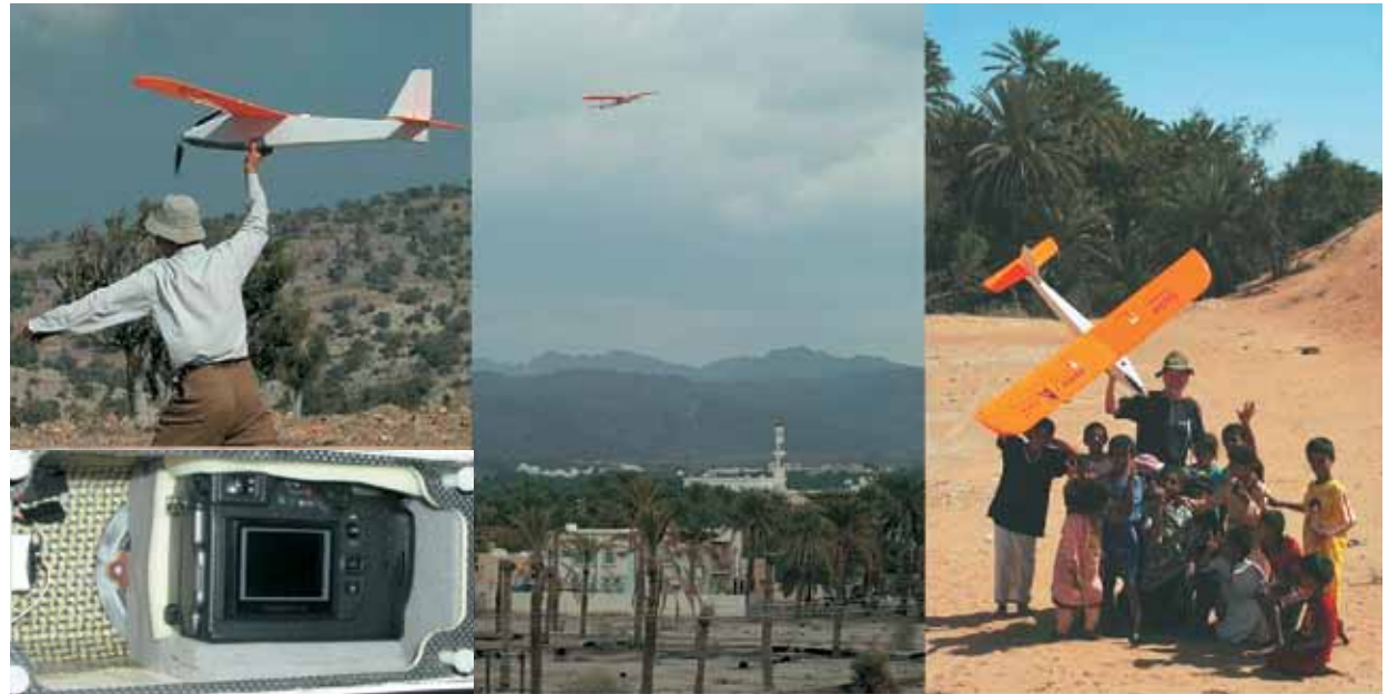
Figure 2. Custom-made, remotely controlled plane equipped to take high resolution aerial photographs of different types of oases in Oman and detail of the digital camera system used.
